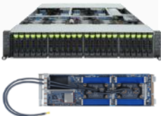
Direct Liquid Cooling
